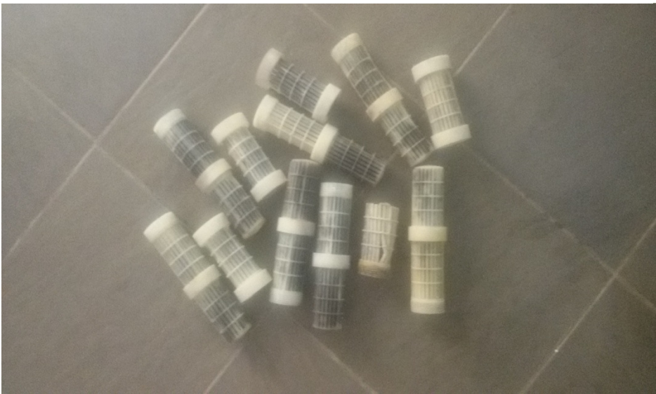
Replacing Lateral Diffuser Nozzles
